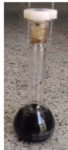
Fig. 1. The stable GO suspension after ultra-sonication process.
