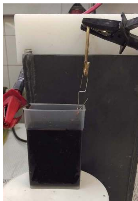
Fig. 2. The anodic electrophoretic deposition process of GO on Cu foil.
